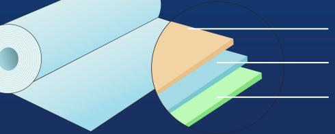
Aluminum Foil High Bond Adhesive Lamination Mylar Film
